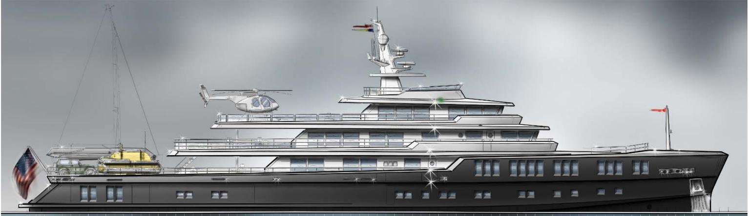
prominent bow and double-chine hull that is capable of handling rougher than normal conditions, while keeping decks dry. The exploration deck has room for two submarines, a quick deployment tender and two jeep style vehicles. A large enclosed garage houses two further limousine style
