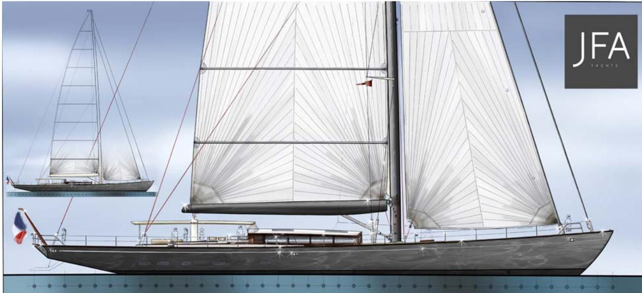
yacht's bow and uninterrupted views down each side of the deck saloon, the amidships position of the helm stations have permitted space for a 14m long aft-deck.
