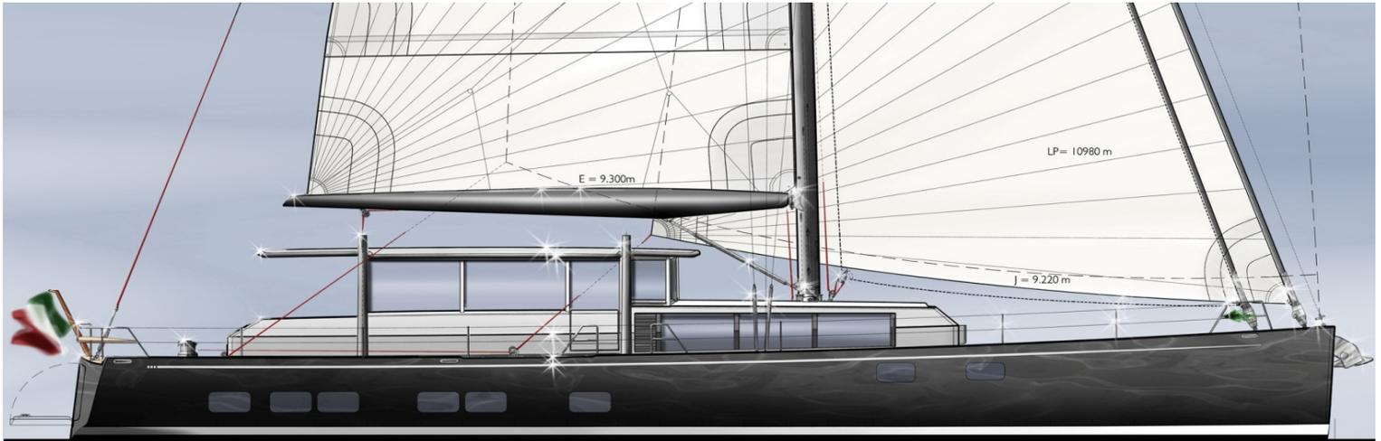
The powerful hull includes a wide beam that extends fully aft, wide transom and flat underwater profile for stability and good downwind performance. The rig comprises a fully-battened main with 'Park Avenue' boom and lazy-jacks system. The sail plan includes a self-tacking inner staysail, No.1 Genoa and the option of a Gennaker or Cruising Shute flown from the bow.
