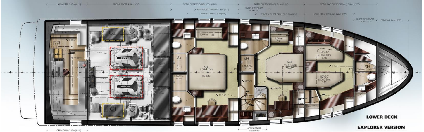
On the Explorer, the space abaft the engines is dedicated to a utility room. She has three full-beam double cabins, which is rare in this size yacht.
