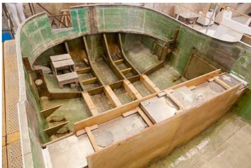
A Menorquin 42 under construction, showing the PVC foam core and the fuel tanks forward of the engine room
