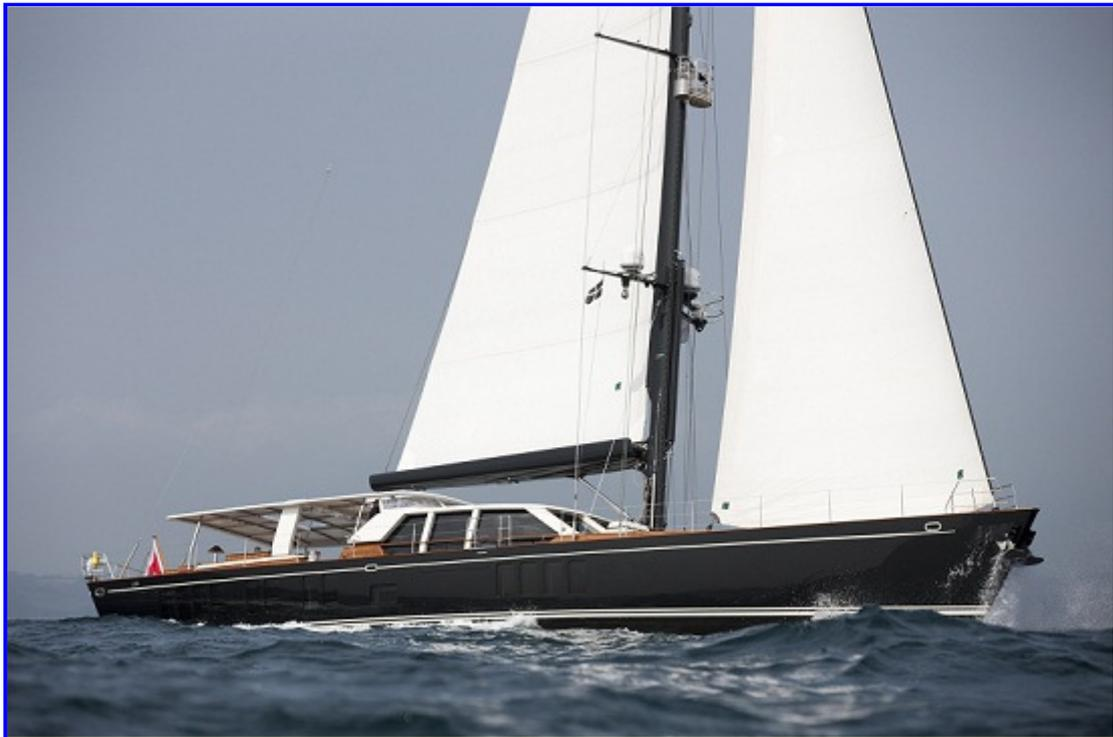
*Akalam* has been specifically designed bearing in mind ease of handling and she is fitted with a JP3 steering system which includes an all-carbon rudder and stock, self-tacking jib and remote control handling of lines and winches. A full onboard control system by SPIN of Barcelona monitors many of the yacht's systems and functions and even controls the bow and stern thrusters, enabling a turning ability that is alike that of a helicopter, using a joystick in the narrowest of spaces.
